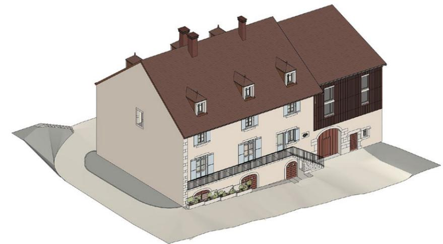
▶ EXEMPLE DE MODELE 3D D'UN BÂTIMENT RÉALISÉ À PARTIR D'UN NUAGE DE POINTS RELEVÉ PAR L'ATELIER DU SURAN
